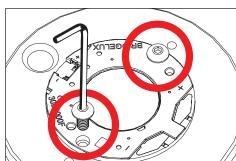
Spread thin, even layer of thermal paste on back of new LED module. Place new LED module onto heatsink, lining up module with holes for screws. Tighten two (2) #4-40 screws using a 1/16" allen wrench to secure LED module to heatsink.
