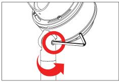
Use a 5/32" allen wrench to loosen #10-32 stainless steel black oxide socket head cap screw at the knuckle for vertical aiming purpose.
