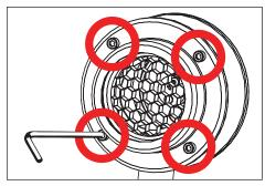
Use a 9/64" allen wrench to loosen four (4) #8-32 stainless steel socket head screws to remove lens bezel.
