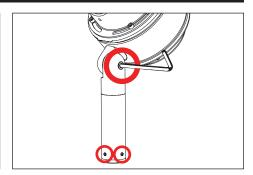
4. Tighten two (2) #8-32 stainless steel set screws on stem to secure horizontal aiming position.
