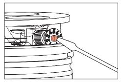
With small flat head screw driver rotate Adjust-e-Lume® dial to desired lumen output.
