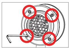
7. Re-install lens bezel. Tighten evenly.
