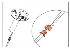
4. Disengage LED board and driver assembly. Replace with new board and driver assembly.
