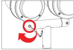
Use a 5/32" allen wrench to loosen #10-32 stainless steel black oxide socket head cap screw at the knuckle for vertical aiming purpose.
