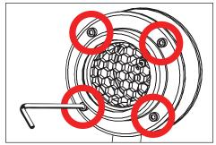
7. Re-install lens bezel. Tighten evenly.
