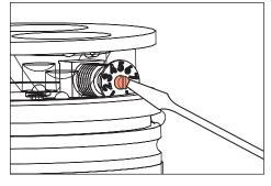
With small flat head screw driver rotate Adjust-e-Lume® dial to desired lumen output.
