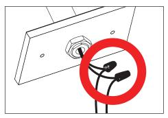
Mount fixture onto suitable enclosure according to designed lighting plan. Use locknut to secure.
