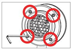
Use a 9/64" allen wrench to loosen four (4) #8-32 stainless steel socket head screws to remove lens hezel
