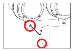
Tighten two (2) #8-32 stainless steel set screws on stem to secure horizontal aiming position.
