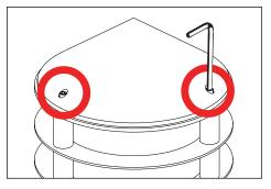
Loosen three (3) captive #10-24 screws on cap with a 1/8" allen wrench.
