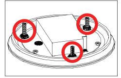
secure the fixture mounting base assembly using three (3) 5/16-18 nuts.
