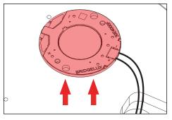
Carefully remove LED module from heatsink.
