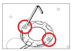
Loosen, then remove two (2) #4-40 screws from LED module using a .050" allen wrench.
