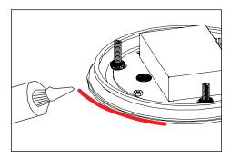
Place a bead of silicone-based sealant (not included) around the mounted plate to create a watertight seal
