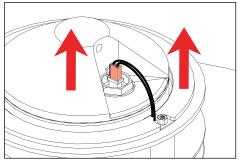
2. Detach heatsink from fixture body via quick 3. disconnect.
