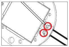
Use small pick tool to push connector off LED board through two small slots behind connector. 5. Once loose, lift connector upwards and off board.
