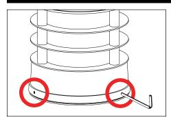
Loosen three (3) 1/4-20 set screws using a 1/8" allen wrench. Lift fixture assembly from base plate assembly.
