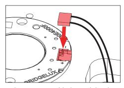
Press connector straight downwards into slot on module to snap into place.
