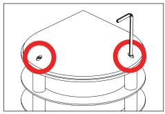
Attach heatsink to fixture body via quick disconnect. Line up on spacers.
