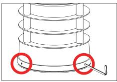
Slide fixture assembly over mounted base plate assembly. Lock in place with three (3) 1/4-20 set screws using a 1/8" allen wrench. Ensure fixture is completely seated.
