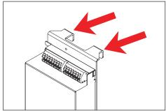
Driver bracket should hang off small horizontal interior bar inside pole near hand hole. Use two hooks on bracket to hang on interior bar.
