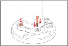
Close hinge pole, then secure to base with three (3) 1/2" I.D. flat washers, split lock washers and three (3) 1/2"-13 stainless steel bolts using an adjustable crescent wrench.
