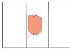
Open hand hole as per pole manufacturer's instructions, then pull primary branch circuit wiring through conduit to splice location and pull down fixture leads from installed pole top.
