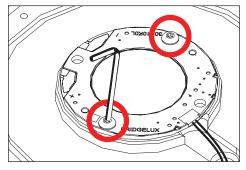
Loosen two (2) #4-40 button head screws with a 1/16" allen wrench.
