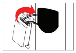
Place connections and driver on bracket into pole through hand hole (for use with 3"x5" hand hole).
