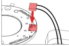
8. Press connector straight downwards into slot on 9. module to snap into place.
