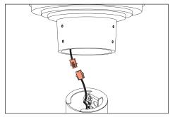
Make secondary connections via quick disconnect from driver secondary side to fixture secondary
