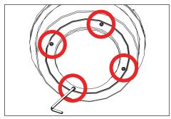
Place dome lens onto heatsink. Tighten four (4) #4-40 socket head set screws on side of dome lens optic holder using a 3/32" allen wrench.
