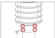
Slide fixture over pole top. Secure with six (6) 1/4-20 socket head set screws using a 1/8" allen wrench. Make sure the fixture is completely seated. Do not overtighten.
