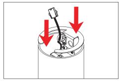
Place connections and driver on bracket into pole. Rest bracket on pole top or tenon.
