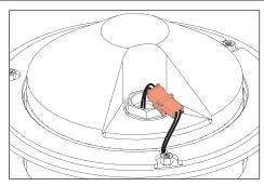
Loosen three (3) captive #10-24 socket head 2. Disconnect quick disconnects at top of heatsink.
