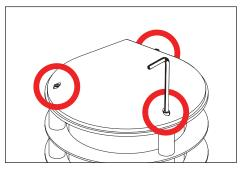
screws on cap with 5/32" Allen wrench.
