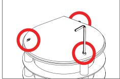
Attach cap with securing three (3) #10-24 socket head screws using a 5/32" allen wrench.
