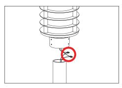
Make watertight connections using waterproof wire 8. connectors to connect fixture leads to secondary leads from driver. Leave length for future service. See wiring diagram.
