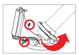
Place driver, bracket and connections into pole. Hinge pole back to upright position. Connect secondary wiring to secondary side of driver. Pull secondary wiring to top of pole. Length of secondary wiring will vary with height of pole. Leave length for future service.
