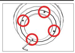
Loosen four (4) #4-40 socket head set screws on side of dome lens optic holder using a 3/32" allen wrench. Gently remove dome lens.
