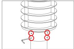
Secure with six (6) 1/4-20 socket head set screws using a 1/8" allen wrench. Make sure the fixture is completely seated. **Do not overtighten.**
