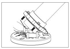
Hinge pole open for access to conduit and branch circuit wiring. Pull branch circuit wiring and dimming controls to splice location.
