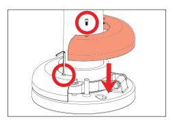
If pole comes with cover, place cover on base of pole. Secure with four (4) 1/4"-20 hex screws using a 3/16" allen wrench.
