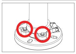
Remove base cover (if required). Open hinge base on pole by loosening three (3) 1/2"-13 stainless steel bolts using adjustable crescent wrench.
