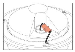
10. Attach heatsink to fixture body via quick disconnect. 11. Line up on spacers.
