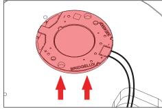
5. Carefully remove LED module from heatsink.
