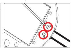
Use small pick tool to push connector off LED board through two small slots behind connector. Once loose, lift connector upwards and off board.
