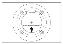
To assure proper operation of the hinge mechanism. The electrical supply conduit must not project more than 1-1/2" above the surface of the concrete.
