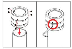
Install tenon (provided with fixture ordered separately) onto the pole top. Tighten six (6) 1/4"-20 set screws using a 1/8" allen wrench until tenon is secured.
