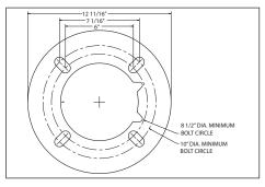
Mounting base is 12-11/16" round with a bolt circle of 8-1/2" to 10" in diameter.
