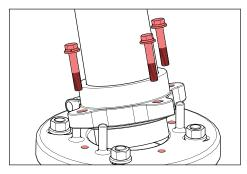
To tilt pole over hinge base, loosen the three (3) 1/2"-13 stainless bolts. Carefully lower pole into a resting position.
