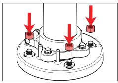
Secure pole base to anchor bolts using provided hardware with anchor bolt kit. Tighten securely to prevent hardware from loosening.
