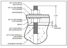
Install anchor bolts according to detail to allow pole leveling. Use caution when setting anchor bolts. Bolts must be vertically straight.
