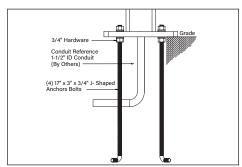
Dig hole for conduit installation and deep enough for anchor bolts and concrete footing. See anchor bolt detail step.
