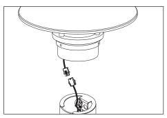
Make secondary connections via quick disconnect from driver secondary side to fixture secondary side.
