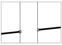
Install provided Anchor Rod into pole through hole.
