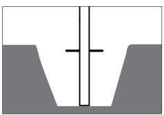
. Place pole over installed conduit. Pull branch 6. circuit wiring through pole and out the top.
