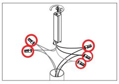
Pull primary branch circuit wiring up to driver bracket location at top of pole. Pull incoming dimming controls to top of pole. Feed through strain relief.
