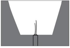
Pole may be directly stubbed into through footing with conduit. Install conduit for branch circuit wiring centered with pole position.
