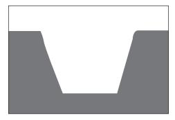
Determine installation location according to lighting plan. Dig hole a minimum of 36" deep and 14" wide. Suitable enough to provide clearance of anchor rod, and proper anchorage for pole.
