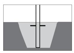
For concrete installation: Fill the hole around the base of pole 24" below grade with clean fill dirt and tamp carefully to prevent further settling. Pour concrete and finish as required flush with finished grade.
