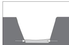
Per DIG-IT Guide, backfill the bottom of pole and bottom of hole with sand for drainage.
