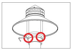
Slide fixture over pole top. Secure with four (4) 1/4-20 screws using a 1/8" allen wrench. Make sure the fixture is completely seated. Do not overtighten.
