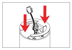
Place connections and driver on bracket into pole. 5. Rest bracket on pole top or tenon.
