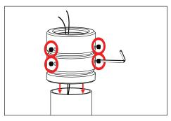
Install tenon adapter provided onto pole top. Tighten six (6) 1/4-20" set screws using a 1/8" allen wrench until tenon is secured.
