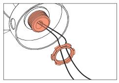
Mount knuckle onto canopy by securing 1/2" NPS stem with provided locknut.
