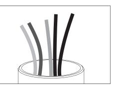
5. Pull primary branch circuit wiring and any additional dimming controls or other wiring necessary for installation.
