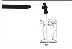
Remove patented knockout(s) as necessary from the inside of the UPM housing. Leave remaining unused knockouts in place to maintain seal.
