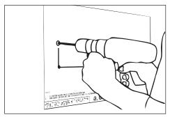
Drill holes into surface for ¼" fasteners on locations 3. required for mounting via tabs.
