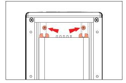
Remove two (2) #8-32 screws in UPM housing using phillips screwdriver.
