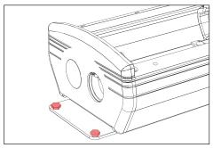
Attach the UPM housing at mounting brackets with 1/4" fasteners. Use suitable mounting hardware for surface.
