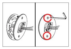
Feed branch circuit wiring and dimming control wiring through mounting plate with CamLock assembly. Attach mounting plate with supplied two (2) #10-24 stainless steel hex drive fasteners to universal ring using a 1/8" allen wrench.
