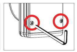
10. Make sure UPM housing gasket is free of any dirt or debris. Attach the faceplate by tightening the six (6) #10-24 captive screws evenly using a 1/8" allen
