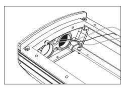
Pull branch circuit wiring and dimming control wiring necessary for installation.
