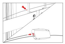
Thread safety cable through hole on the back of the UPM housing. Feed safety cable through opposing ends of the connector. Pull on wires to assure the connection is secure. Leave enough slack in safety cable for tree growth. Adjustments can be made by pressing release spring with a pin or a 3/64" allen tool.
