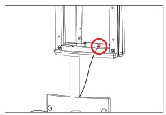
8. Attach tether wire under screw head at the base of the UPM housing and tighten. Slowly lower the faceplate until tether is taut.
