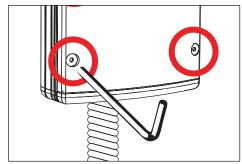
12. Make sure UPM housing gasket is free of any dirt or debris. Attach the faceplate by tightening the six (6) #10-24 captive screws evenly using a 1/8" allen
