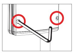
Slide driver feet under two screws in UPM housing and tighten screws using phillips screwdriver.
