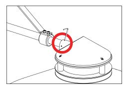
Slide fixture body onto stem, then secure by tightening two (2) #8-32 set screws with a 5/64" 4. allen wrench.
