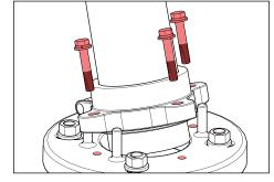
To tilt pole over hinge base, loosen the three (3) 1/2"-13 stainless bolts. Carefully lower pole into a resting position.
