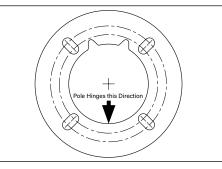
4. To assure proper operation of the hinge mechanism, the electrical supply conduit must not project more than 1-1/2" above the surface of the concrete.
