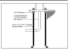
2. Dig hole for conduit installation and deep enough for anchor bolts and concrete footing. See anchor bolt detail step.
