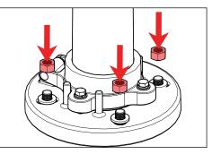
Secure pole base to anchor bolts using provided hardware with anchor bolt kit. Tighten securely to prevent hardware from loosening.
