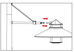
3. Connect secondary leads in stem with secondary leads from fixture body with quick disconnect. Connect remote driver secondary wiring to fixture leads using watertight wire connectors (not included) as per NEC. Place wiring and connections
