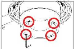
Loosen four (4) #4-40 set screws on dome lens optic holder using a 0.050" allen wrench. Gently remove dome lens optic and optic holder.
