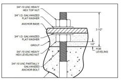
Install anchor bolts according to detail to allow pole leveling. Use caution when setting anchor bolts. Bolts must be vertically straight.
