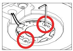
4. Loosen two (2) #4-40 screws with a 0.050" allen wrench. Gently pull optic holder off heatsink.
