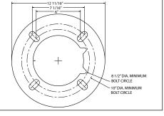
1. Mounting base is 12-11/16" round with a bolt circle of 8-1/2" to 10" in diameter.
