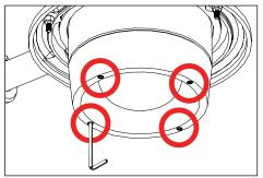
Place dome lens and optic holder back onto cap. Tighten four (4) #4-40 set screws on dome lens optic holder using a 0.050" allen wrench.
