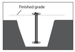
Install anchor plate and bolt assembly flush and level with the finished grade.
