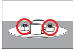
The fixture may be installed by removing the two (2) 1/4-20 nuts and re-using them with a 7/16" wrench to secure the fixture mounting base assembly. See fixture installation sheet(s) for additional information.
