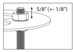
Adjusted anchor rods to project no more than 5/8" with a variance of + or - 1/8" above the anchor plate after installation. The two (2) 1/4-20 nuts on top of the plate may be left in place while concrete is poured.
