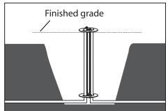
Run conduit inside of the anchor plate center holes prior to pouring concrete. Conduit installation through bottom plate is optional.
