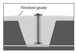
With the conduits in place and the anchor plate properly positioned, secured and leveled, concrete may be poured.
