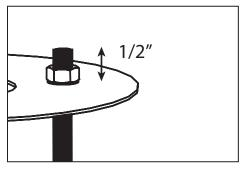
Adjusted anchor bolts to project at least 1/2" but no more than 5/8" above the anchor plate after installation. The four (4) 1/4-20 nuts on top of the plate may be left in place while concrete is poured.
