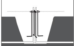
Run conduit inside of the anchor plate center hole prior to pouring concrete. The conduit may project above the finished surface of the concrete by 3/8" maximum.
