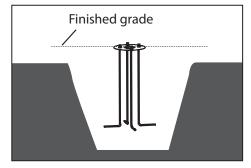
Install anchor plate and bolt assembly flush with the finished grade.
