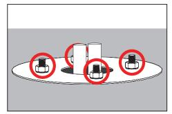
The fixture may be installed by removing the four (4) 1/4-20 nuts and re-using them with a 7/16" wrench to secure the fixture mounting base assembly. See fixture installation sheet(s) for additional information.
