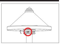
5. Replace shade. Tighten three (3) #8-32 set screws on shade assembly using a 9/64" allen wrench.
