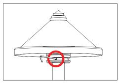
Loosen three (3) #8-32 set screws on shade assembly using a 9/64" allen wrench and remove.
