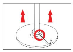
Loosen set screw using a 5/64" allen wrench on locking ring. Slide locking ring and canopy cover up.
