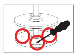
Attach mounting plate to suitable enclosure in final fixture location according to designed lighting plan using appropriate hardware (hardware not included). Seal as per NEC.
