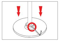
Slide canopy cover and locking ring over mounting plate and tighten set screw using a 5/64" allen wrench.
